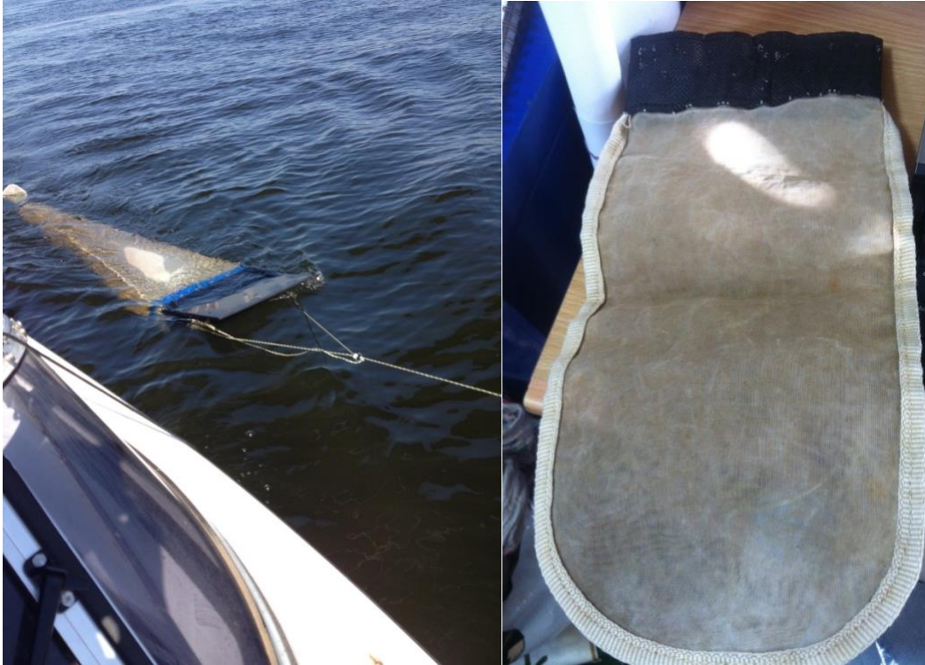
Figure 3: A. Manta net deployed on side of Yarra Riverkeeper vessel. B. Codend used to capture microplastic samples.
