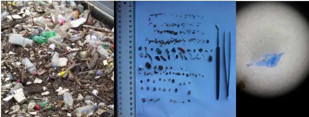
Figure 4: A. Litter caught in Yarra River boom traps breaks up into millions of microplastics. Photo courtesy of Heidi Taylor. B. Microplastics collected in the Yarra River as part of the Trawl program. C. Image of <1mm microplastic item sourced in the Yarra River
